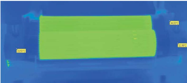
These two new top rollers also run about 2 minutes: The bearings are still at room temperature. The top rollers are beginning to warm up.
