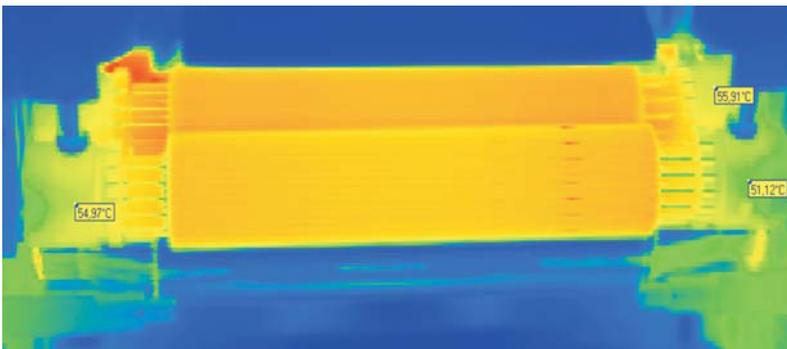
The final temperature of the new top rollers is about 10°C lower than with conventional top roller coatings. This is achieved by heat dissipation to the bearings. They are about 25°C colder than with conventional system.
