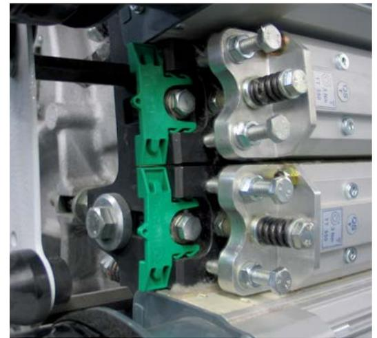
T-Con-Spacers are inserted between assembly bend and fixed carding segment and automatically fixed.
