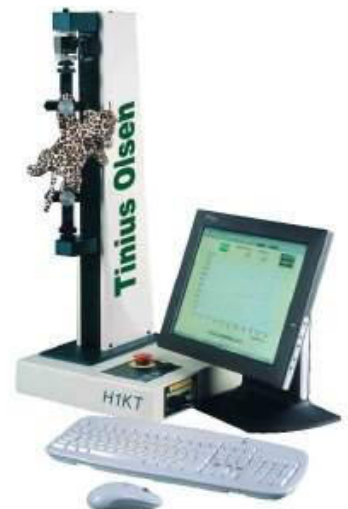
Model H1KT testing a stuffed toy
