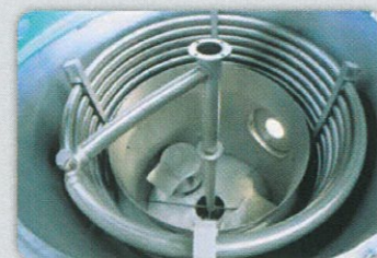
Primary distillation unit: pre-heating
