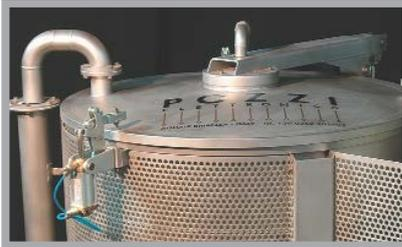
Electro-polishing of the inner surfaces of the tank that eliminates the sticking of the dyestuff to the wall.
