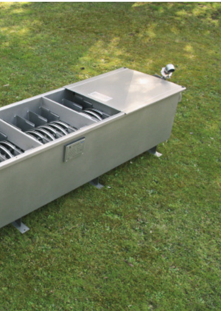
Heat recovery from a discontinuous process: exchangers installed in a water treatment plant
