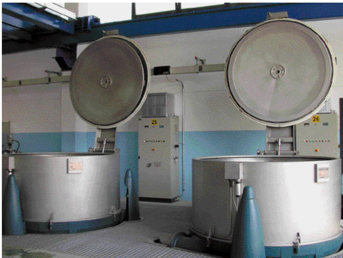
basket. At the end of the hydro extracting operation, the unloading comes about in the same way but with an inverted rotation.
